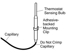
Figure 52 - Positioning the Thermostat Sensing Bulb in the Vertical Position with the Capillary at the Bottom
